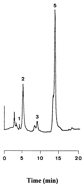
Figure 3. Chromatogram of a sample of sea water containing the metabolites generated by the biodegradation of LAS. Injection of 10 \mu L. Detection, UV at 215 nm, 0.05 AUFS. The separation conditions and the number of peaks as in Figure 2 A. The content of each metabolite is reported in Table 5.
